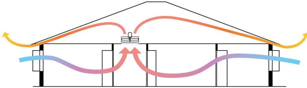
The fan moves about 6 cubic metres of air a second, far more than an air conditioner. Even though the temperature of the air rises by only three degrees or so, it removes an enormous amount of heat all through the night. The cooler air removes unwanted heat from the structure of the home: the walls, ceilings, furnishings and floors.
